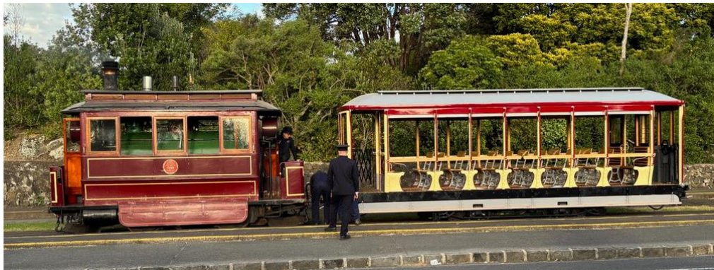
MOTAT's newly restored Wanganui trailer No 21 was tested behind Baldwin steam motor No 100 on Tuesday 17 March, before its official launch the following Sunday. (David Cawood)
